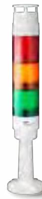
Order no.: CT5-Q06 Colours: red/amber/green Function: LED steady beacon, Piezo buzzer module, one of eight tones can be selected with a dip switch Nominal voltage: 24 V DC Type of mounting: Tube mounting (100 mm tube length)
