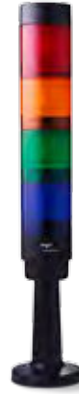
Order no.: CT5-Q05 Colours: red/amber/green/blue Function: LED steady beacon Nominal voltage: 24 V DC Type of mounting: Tube mounting (100 mm tube length)
