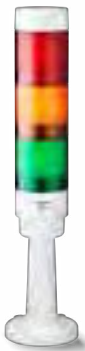
Order no.: CT5-Q03 Colours: red/amber/green Function: LED steady beacon Nominal voltage: 24 V DC Type of mounting: Tube mounting (100 mm tube length)
