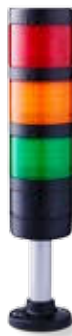
Order no.: PC7-Q01 Colours: red/amber/green Function: LED steady beacon Nominal voltage: 24 V AC/DC Type of mounting: Tube mounting (100 mm tube length)
